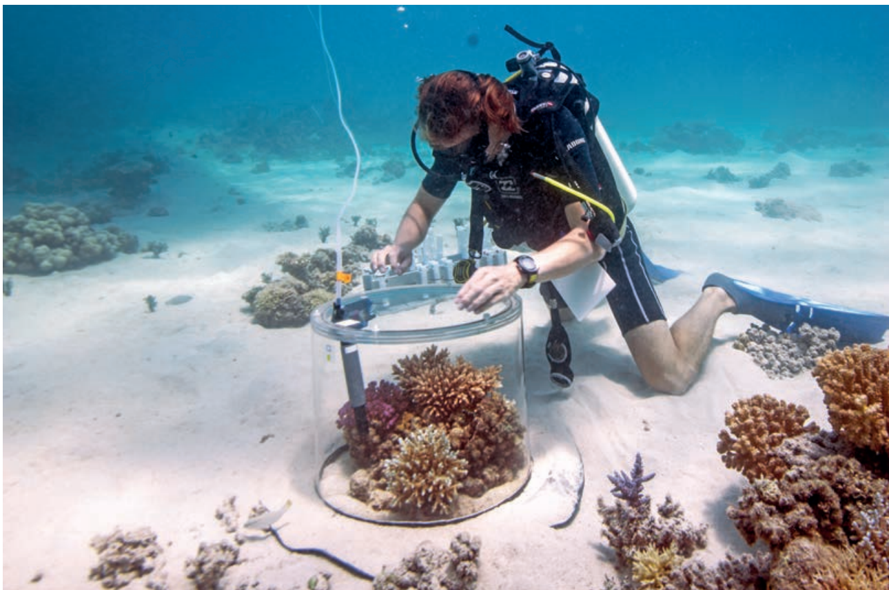
Fig. a: Design of a field study with a transparent plastic chamber in order to continuously measure the cycle of materials between the water column and the benthic organism communities of a coral reef in the Red Sea.
